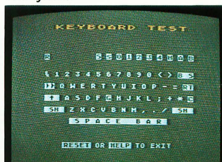
SCREEN 4 During the keyboard test, press keys to see that they change their screen images.
